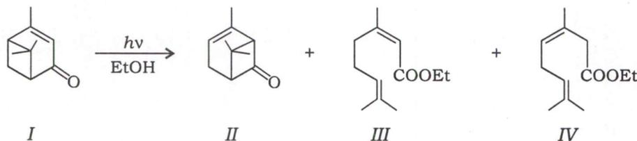
Ethanol solution of compound I on irradiation leads to the formation of compounds II, III and IV. The resulting reaction mixture exhibits bands at 1787, 1740, 1715 and 1685  $\text{cm}^{-1}$  for  $\nu_{\text{C}=\text{O}}$ . Assign these  $\text{C}=\text{O}$  stretching frequencies to the corresponding compounds giving reasons :
