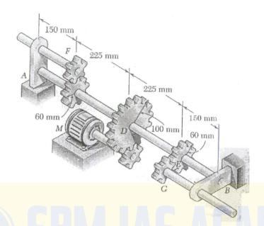
A solid shaft AB rotates at 450 rpm and transmits 20 kW from the motor M to machine tools connected to gears F and G. A power of 8 kW is taken off at gear F and 12 kW is taken off at gear G. The allowable shear stress is 55 MPa. Determine the smallest permissible diameter of the shaft AB.
