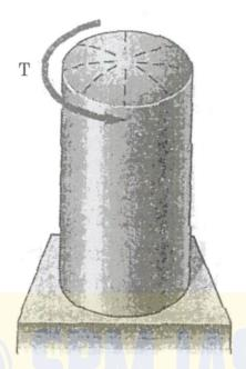
A tank shown in the figure is filled with compressed air under pressure of 8 MPa. A torque of magnitude T = 12 kNm is applied at the end. The tank has an inner diameter of 180 mm and thickness of wall 12 mm. Determine the maximum normal stress and maximum shearing stress in the tank considering the cylinder is thin.
