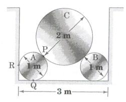
A cylinder C weighing 1000 N is supported by two cylinders A and B weighing 500 N each as shown in the figure. Calculate the contact forces at P, Q and R.
