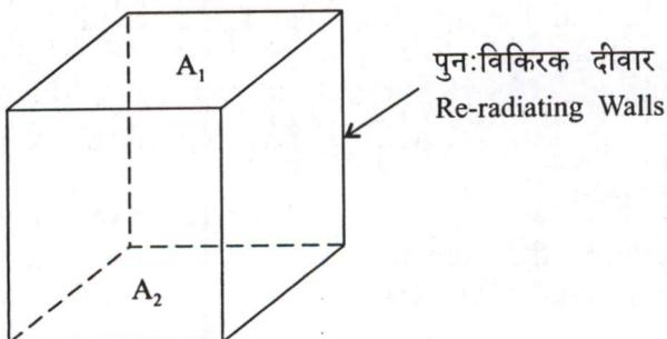
Show that the effective conductance, ( $A_1 \bar{F}_{12}$ ) for two black, parallel plates of equal area connected by re-radiating walls at constant temperature is
